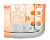
CPR Detection - the iPAD SP1 detects if CPR is being performed when appropriate
